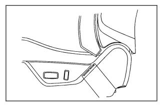
If your seats have power reclining seatbacks, use the vertical power seat control located on the outboard side of each seat.
